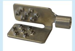
The crimp tool compresses the connector to the round feed cable and clamps the teeth of the crimp onto the copper tape. There are three different types of crimps, two for different gauge wires (10-12AWG and 14-16AWG) and one for extending lengths of copper tape (Termi-foil splice crimp).
