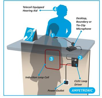
To use the system a hearing impaired customer needs only to switch the hearing aid to the 'T' position. Expensive receivers are not required and users don't suffer the inconvenience of asking for and wearing a headset that marks them out as hard of hearing.
